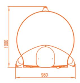
Cooking chamber: Dome and hearth in chamotte. Diameter 700mm thickness 40mm
